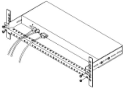
*Figure 2: Assembling rack cable support*
