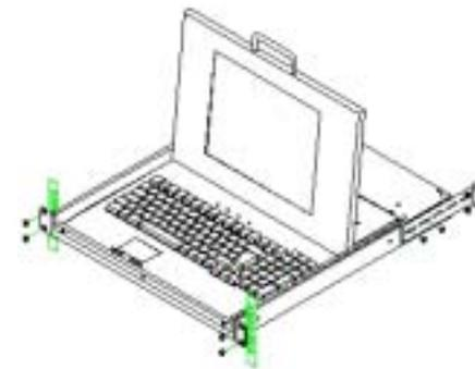
Figure 1: Attaching rack mount bracket
