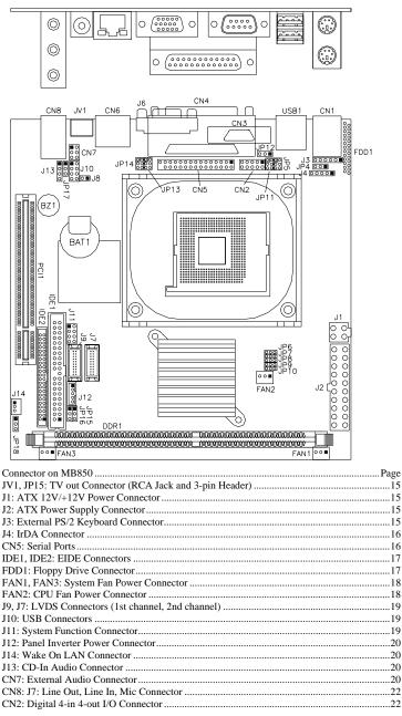
JV1, JP15: TV out Connector (RCA Jack and 3-pin Header)
