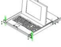
Figure 2 shows how to assemble rack cable support then screw it to the back and inside the rack cabinet vertical post (optional).
