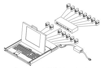
Figure 2: A cascade KVM Switches configuration
