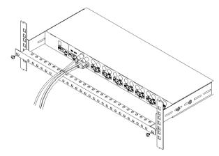
Then, keyboard/mouse/monitor cables can be routed over the cable support. You can use plastic cable ties to bundle and label the cables through the rack cable support holes for easy identification.
