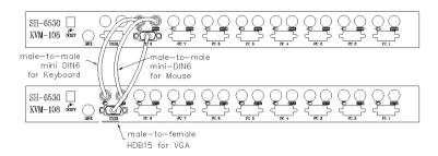
Figure 10: Slave console connection
