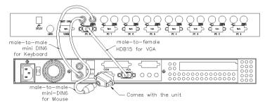
Figure 5: Adapter and serial mouse connection
