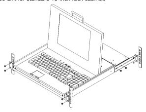
Figure 6: Attaching rack mount bracket
