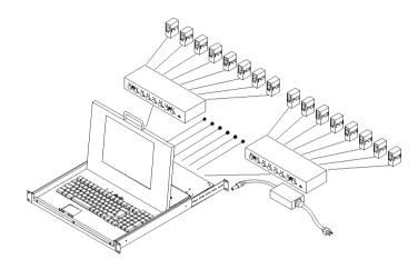
Figure 11: Cascaded 8-port KVM Switches
